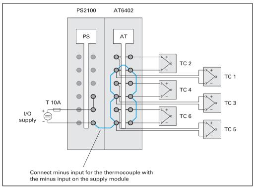
Figure 414: AT6402 - Connection of ceramic heating elements with integrated thermo elements
