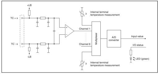
Figure 413: AT6402 - Input circuit diagram
