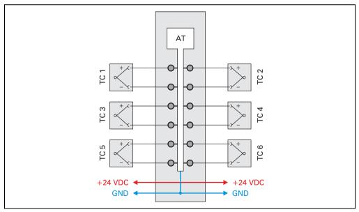
Figure 412: AT6402 - Connection example
