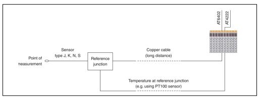
Figure 415: AT6402 - External reference junction for bridging large distances
