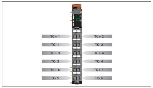
Figure 411: AT6402 - Pin assignments
