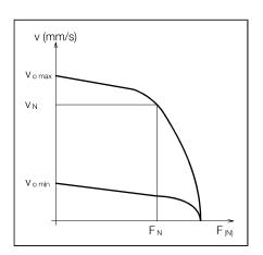
The nominal positioning force  ${\rm F_N}$  of the actuator should exceed the break-away force  ${\rm F_L}$  of the reel.
