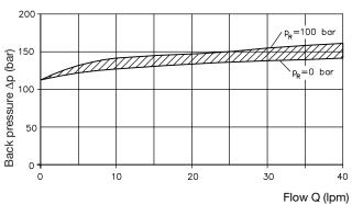
Viscosity during measurements approx. 60 mm<sup>2</sup>/s
